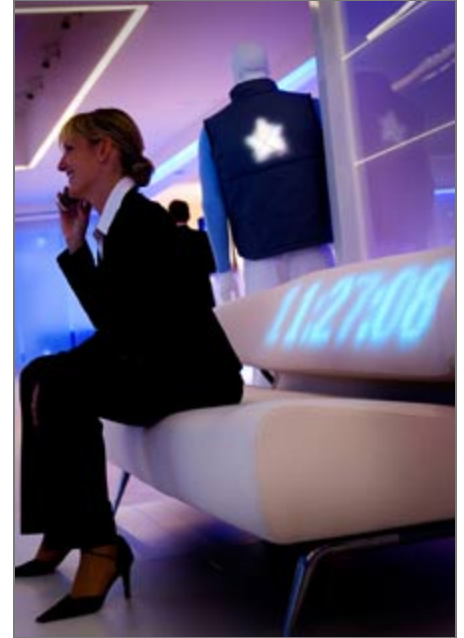
A sofa using Philips' Lumalive textile technology displays the time, while a mannequin in the background sports a jacket with a Lumalive design stitched into it.
